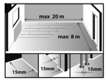
Having established the direction, the width of the room should be measured. This number should then be decreased by 30mm (ie an expansion gap of 15mm at either side), and divided by the board width of the chosen product. This will then give the number of rows of boards to be assembled and the width of the final row.
