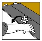
8. Place the board tight to the short end of the previous board and fold down in a single action movement, again ensuring the short joint 'clicks' and locks.
