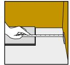
4. At the end of the first row, place a 15mm expansion gap spacer against the right hand wall or skirting board, and measure the length of the last board to fit.
