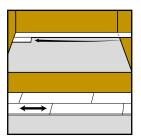
6. Second row. First board, min length 500mm. Use the off cut from the final first row board, (if it is 500mm or longer) to start the second row of boards, Again leave an expansion gap of 15mm against the left hand wall or skirting board. Ensure a minimum 150mm distance between the short end joints of the boards laid in the previous row and the new row being laid.
