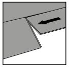
7. Second board second row. Locate the long edge groove of the board onto the long edge tongue of the previously laid row.
