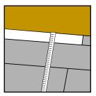
10. Final row. Measure the width of the final row of boards The final row of boards must have a minimum width of 50mm and a minimum 15mm expansion gap must again be left at the edge.
