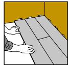
9. After 2-3 rows. Adjust, if needs be the distance between the front wall or skirting and the flooring edge and ensure adequate numbers of 15mm spacers are in place to keep the flooring edge a minimum 15mm away from the wall or skirting at all points along this edge.
