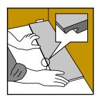
1. First board, first row. Place 15mm expansion gap spacers against the walls or skirting boards at the left hand end, and back long edge, of the first board and position the board end against the wall. The groove on the back edge of the board should be against the spacers on the facing wall.
