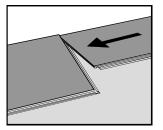
When locating and folding down the board short end joints the PVC locking strip of the 5GC system is automatically pushed across and springs back and locks the two header profiles of the joints together.
